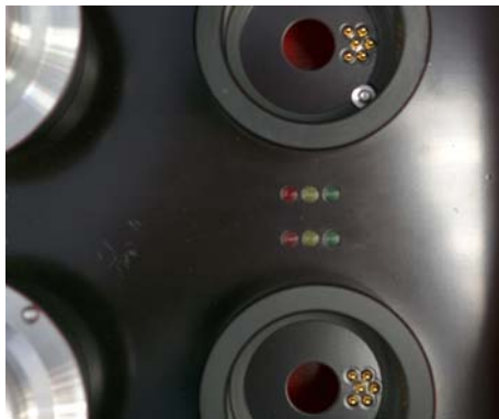
Fig. 27: Signal indicators on the charging adapter - box type
